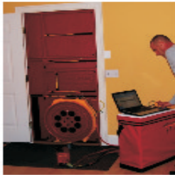
Measures air-leaks that cause Energy loss
